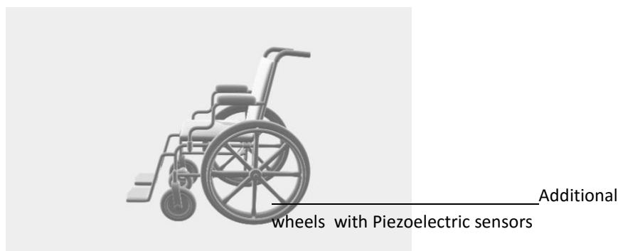
Fig 2.1a 3D model of the piezoelectric wheelchair (Bottom view)
